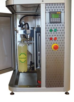
The Somex Co2 Mechanical Shaker is a repetable and robust laboratory or 'at line' device used to accurately determine the dissolved Co2 in a beverage. Constructed almost entirely from Stainless Steel it is ideal for monitoring the Co2 level in carbonated beverages. After each cycle the Temperature and Pressure are displayed on the operator screen which can be used in conjuction with a correlation chart to determine the final Co2 measurement.
